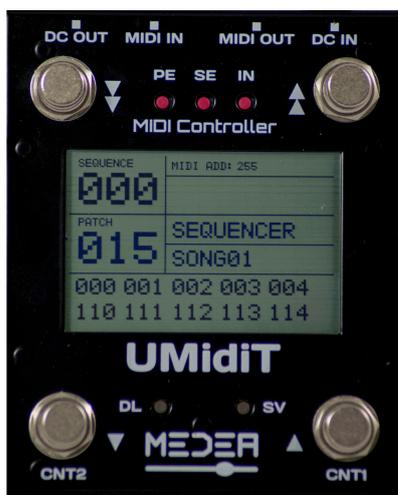
An external power supply must be connected to the **UMIDIT** DC IN connector; the voltage supply must be between 9 and 12 V (MAX) with at least 100mA.
