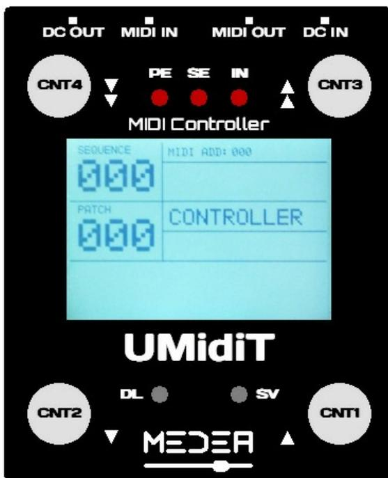
The "PATCH" number is the "Cn" MIDI command that is sent through the MIDI OUT connector. When you use the CNT3 and CNT4 footswitches the Cn command will be sent only after the CNT1 or CNT2 will be pushed. The rightmost digit will be forced to 0.
